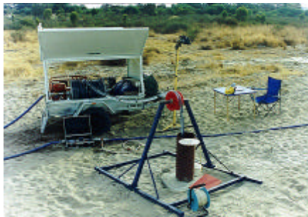
Test pumping equipment
